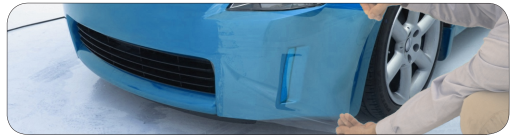
VentureShield™ film being applied to the bumper on this vehicle.
