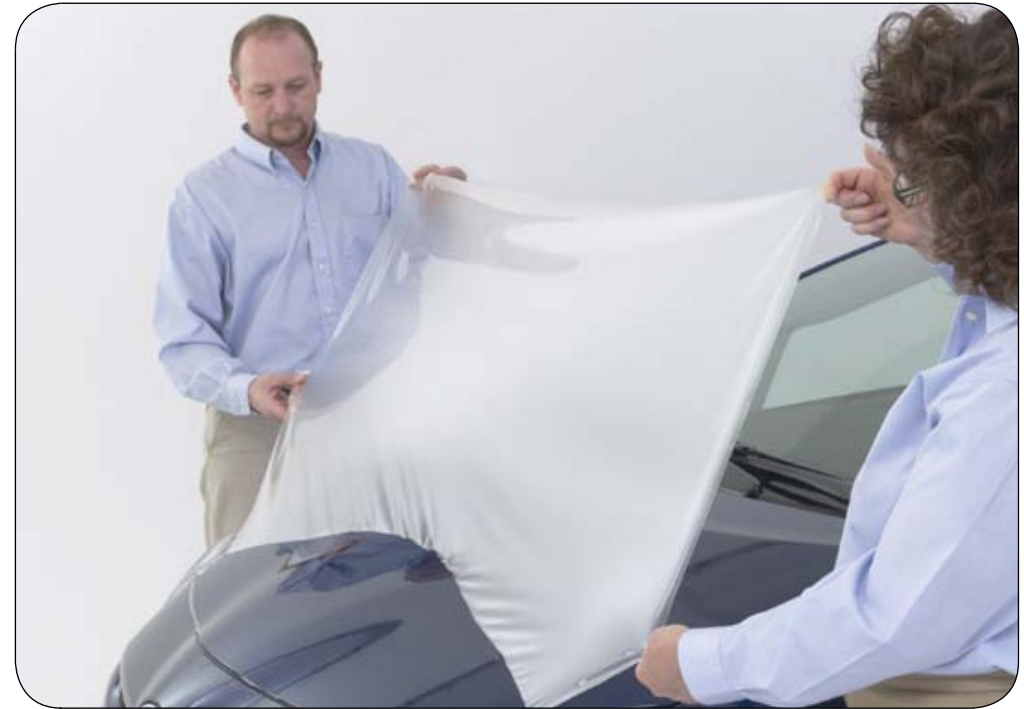
VentureShield™ film is available in 60" width, enabling coverage of the entire hood.
